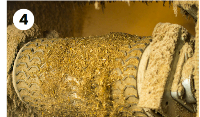
4 Each particle is now coated in mycelium and we break it up into loose particles again
