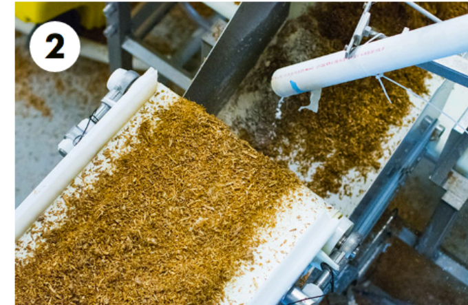
2 Clean the agricultural waste and introduce it to mycelium
