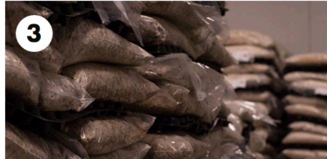
3 Bag this mixture and let the mycelium grow for a few days. The mycelium sees the agricultural waste as food and reaches out to digest it, forming a matrix of white fibers along the way
